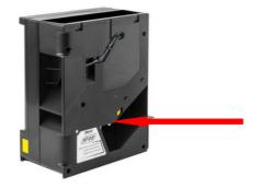
DO ALWAYS CONNECT THE PINPOINTED METAL PLATE OF THE HOPPER TO THE MACHINE GROUND TERMINAL, TO PREVENT ANY POTENTIAL DAMAGE CAUSED BY HEAVY ELECTRO-STATIC CHARGE INTRODUCED WITH THE COINS.
